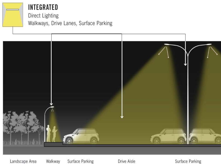
Figure F-7: Lighting Design Requirements-Surface Parking
