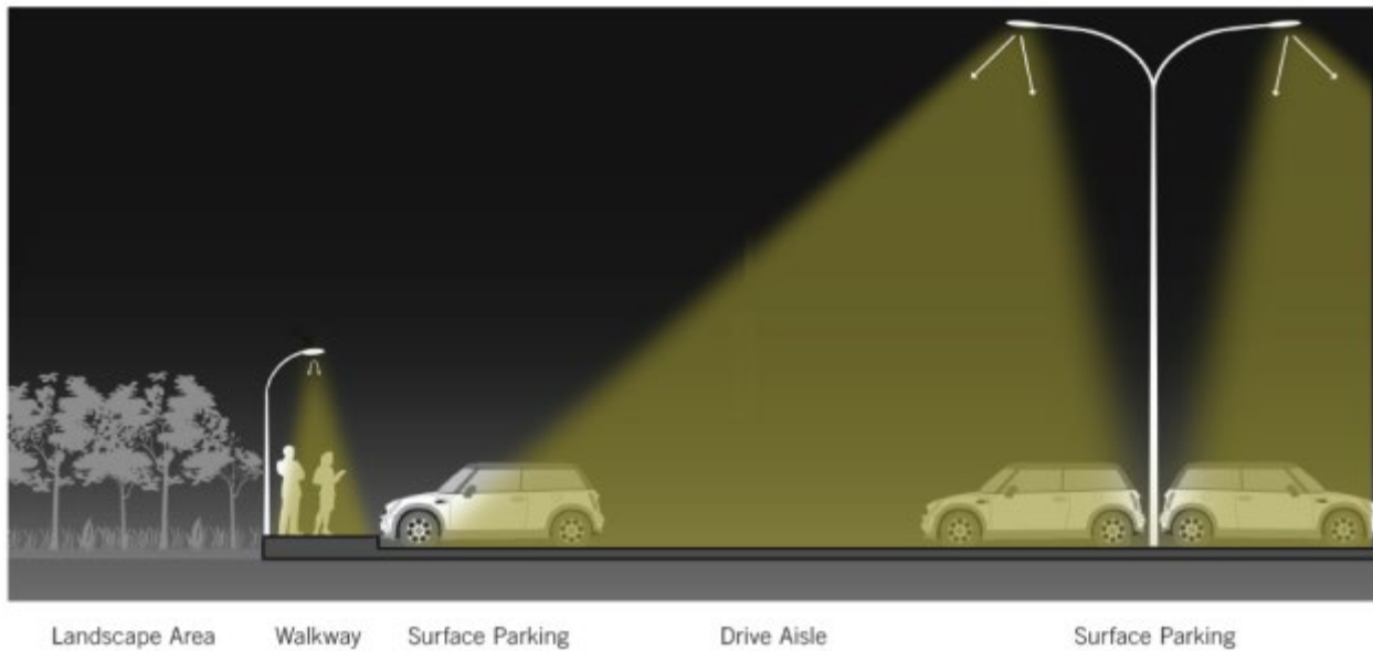
Figure 28: Lighting Design Requirements - Surface Parking
