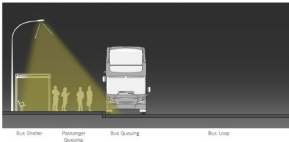
Figure 26: Lighting Design Requirements - Bus Loops
