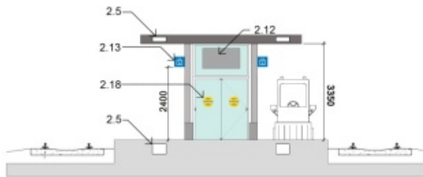
Figure 6: Typical Rail Platform Elevation - Section A
