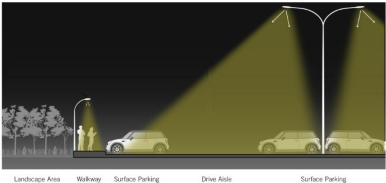
Figure 21: Lighting Design Requirements - Surface Parking
