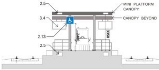
Figure 6: Typical Rail Platform Elevation - Section B
