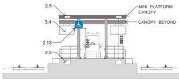
Figure 6: Typical Rail Platform Elevation - Section B
