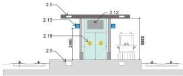
Figure 5: Typical Rail Platform Elevation - Section A
