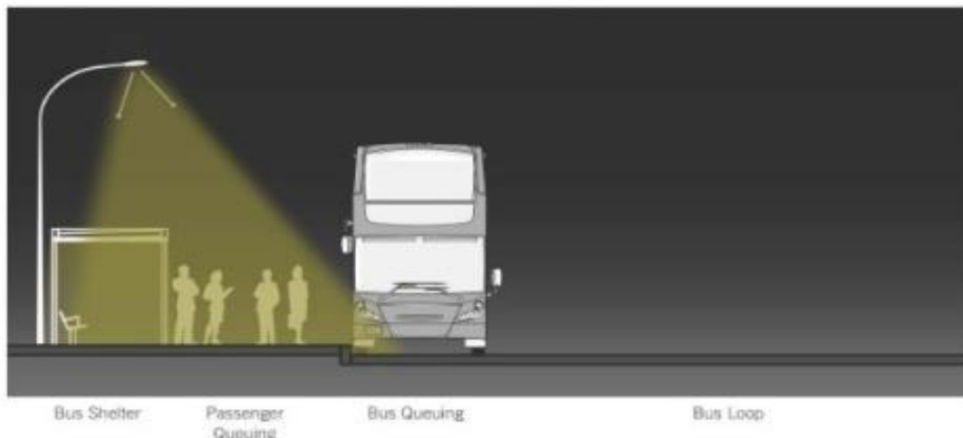
Figure 17: Lighting Design Requirements - Bus Loop
