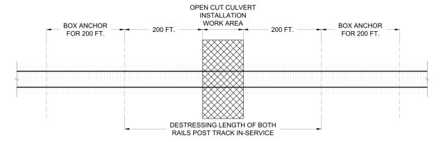
Figure 38-A. Destressing Length for Open Cut Culvert Installations
