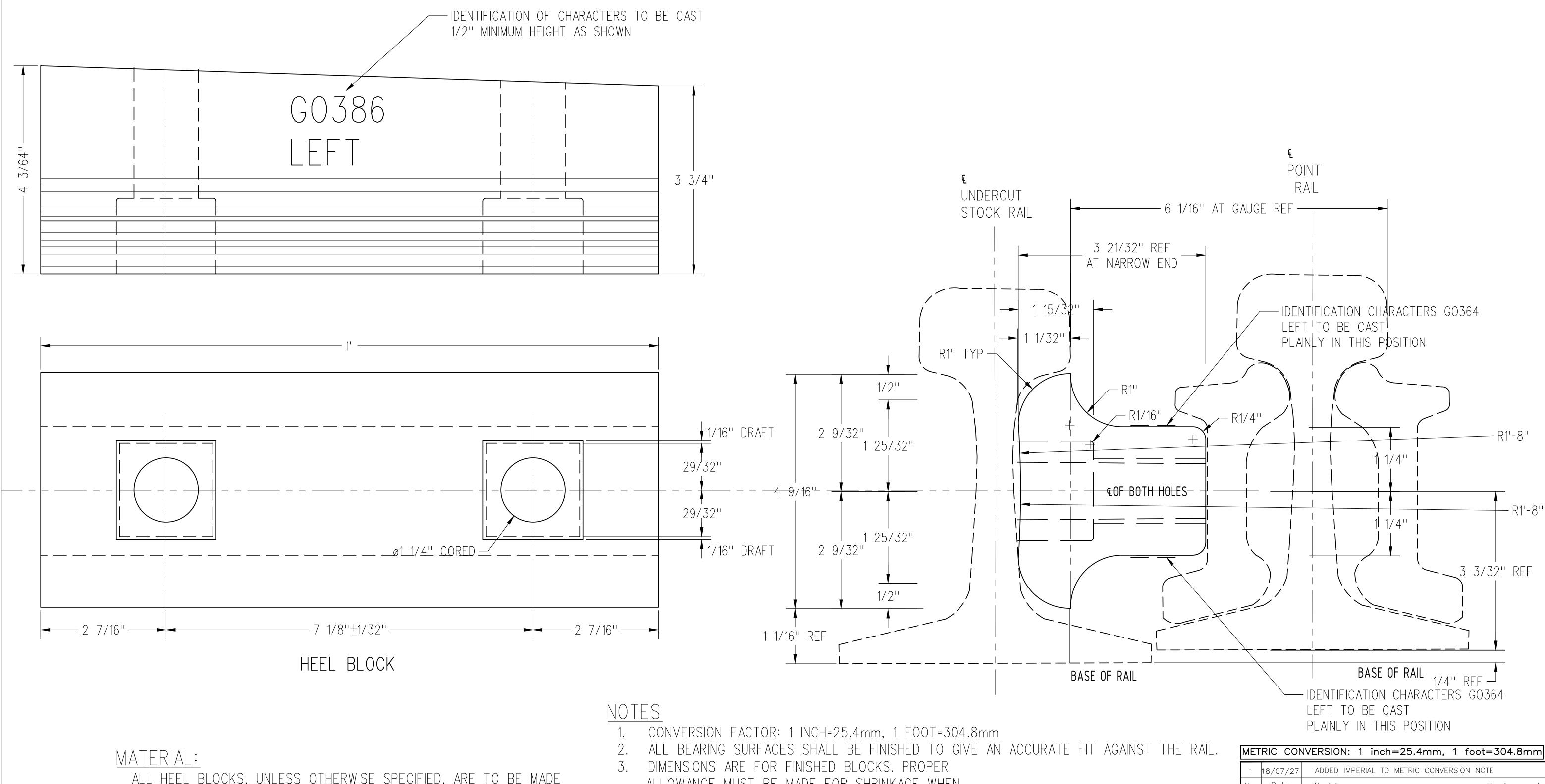
ALL HEEL BLOCKS, UNLESS OTHERWISE SPECIFIED, ARE TO BE MADE IN GENERAL WITH LATEST REVISION OF A.S.T.M. SPECIFICATION FOR: MALLEABLE IRON A47, GRADE 32510 OR DUCTILE IRON A536, GRADE 65-45-12
