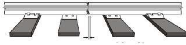
Minimum 1 to maximum 1 1/8 inch. Note: extra preheat for 30 seconds may be required at 1 1/8 inches
