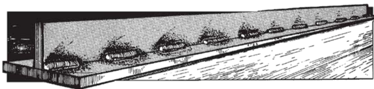
Figure 8.15-Staggered intermittent welds/ chain intermittent welds
