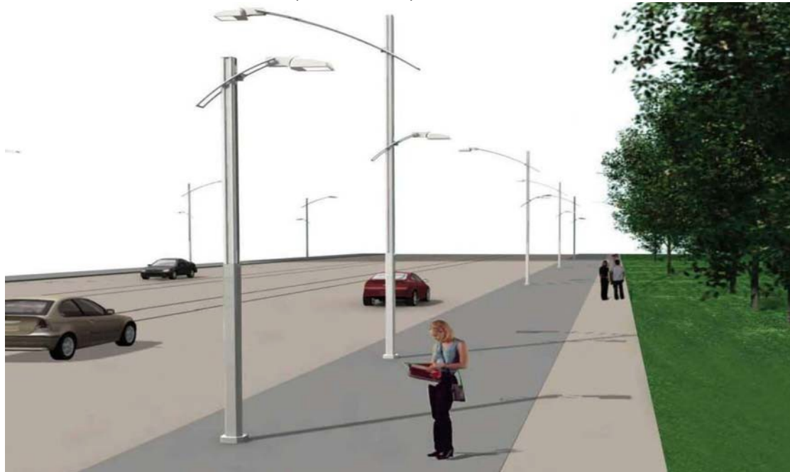
FIGURE C3-1 STREET/PEDESTRIAN LIGHTING SYSTEM (NOT TO SCALE)
