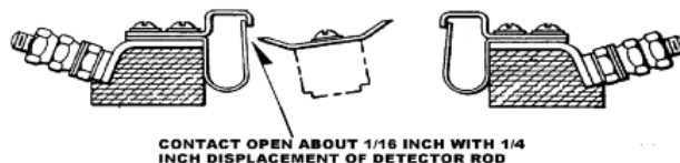
Figure 329(b)(2)- 4: GRS Switch Machine Point Detector Contacts.
