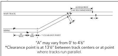
Figure 001-12: Turnout - Where Fouling Protection Not Used
