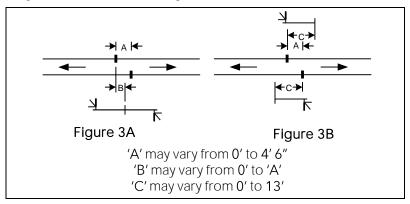
Figure 001-4: Automatic Signal (i.e. Single Approach or Intermediate Signal)
