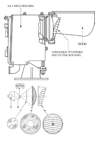
Figure 012-17: GRS TYPE SA-1 LOW MAST SIGNAL WITH STEPPED LENS WITH PHANKILL
