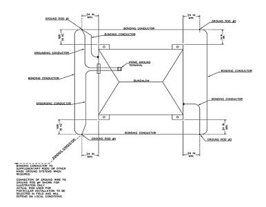
9.3. Made ground systems at cases must consist of at least two ground rods. The ground rods must be bonded together and have two grounding conductors connected to the housing prime ground terminal as shown in Figure 1102-6.
