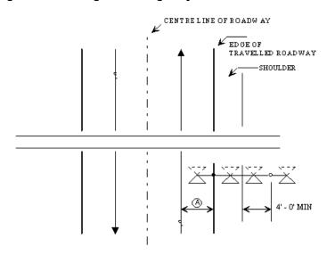
Figure 703-4: Multilane Highway Without Curb
