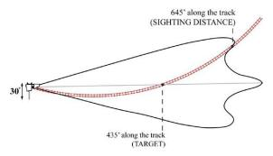
Figure 012-8: VERTICAL MAIN BEAM ALIGNMENT FOR ALL TYPES OF UNITS
