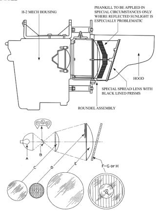
Figure 012-13: US&S TYPE H-2 HIGH MAST SIGNAL
