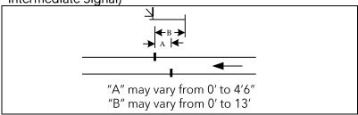
Figure 001-5: Automatic Signal (i.e. Back to Back Approach or Intermediate Signals)
