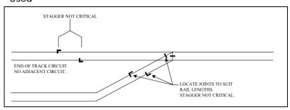
Figure 001-13: Railway Grade Crossing - One Common Rail Track Circuit
