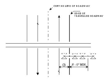
Figure 703-2: Single Lane Highway With Curb
