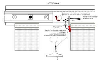
8.2. Figure 007-10: Track Connections – Far Rail, Concrete Tie provides detail on how to attach the far-rail track connections for a concrete tie application.
