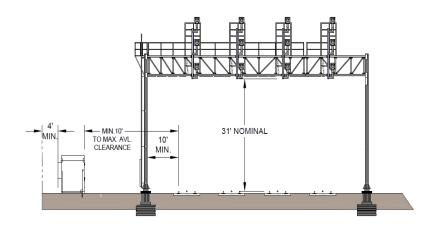
Figure 302-2: Location and Clearance of Signal Cantilever
