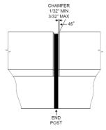
Figure 008- 7: Bevel Around Entire Head Profile
