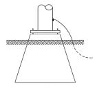
9.7. Made ground systems at transformer and arrester poles must consist of at least two ground rods. The ground rods must be bonded together and have a single grounding conductor connected to the pole top equipment as shown in Figure 1102-10.
