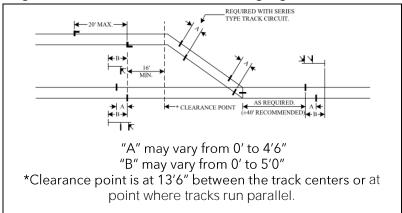
Figure 001-7: Crossover - Main Tacks Interlocked or Non-Interlocked
