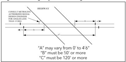
Figure 001-17: Highway Grade Crossing - Electronic Island Circuit
