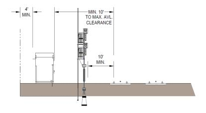
Figure 302-4: Location and Clearance of Wayside Enclosures
