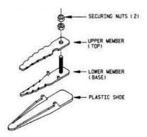
10.3. The 4460-S connector consists of 5 pairs: lower member (base), upper member (top), 2 securing locknuts and a plastic shoe to aid connector insertion and to protect the communication conductors. Rows of teeth on both the top and base members pierce the thin polyolefin film which coats the aluminum shield and bite into the outer polyethylene jacket to provide good-pull-out resistance. Figure 1002-8 illustrates installation of the shield connector.
