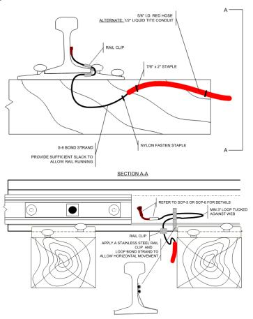
Figure 007-8: Track Connections - Far Rail, Wood Tie
