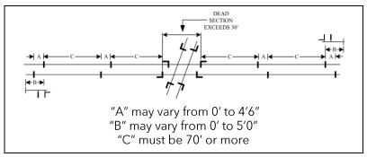
Figure 001-16: Highway Grade Crossing - DC Island Circuit
