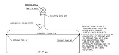
9.5. Made ground systems at WCP radio towers must consist of at least two ground rods placed across from each other with the tower in the middle. The ground rods must be bonded together and have two grounding conductors connected to the tower as shown in Figure 1102-8. The bonding conductor ring must be in a circular pattern.
