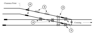
Figure 011-3B: Shunt Fouling - GCWS Non-Signalled Track More Than 300 Feet
