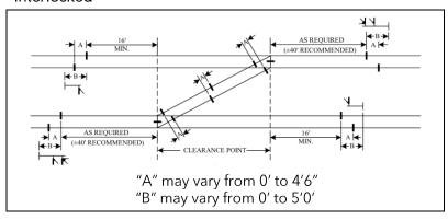
Figure 001-8: Crossover - Main Track to Siding Switch Normally Lined Through on Siding
