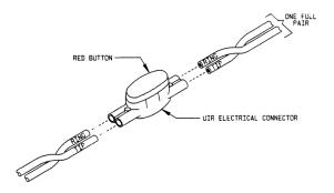
12.2. Scotchlok connectors employ u-shaped elements which are forced down causing the elements to pierce and shear through the conductor insulation. The spring loaded metal fingers of the u-element develop a high contact pressure on the conductor. The u-elements are encased in a Transparent plastic sleeve filled with silicone grease sealant which excludes moisture but will not harm polyethylene or other insulations.
