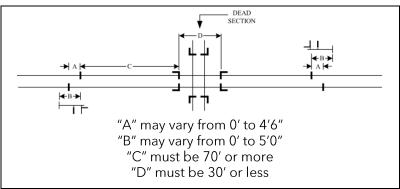
Figure 001-15: Railway Grade Crossing - Trap Circuit for Dead Section Greater than 30'
