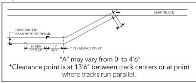
Figure 001-11: Turnout - With Track Shunt
