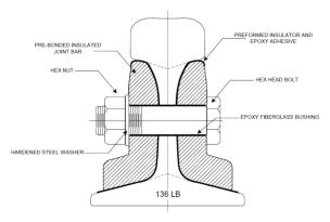
Figure 008-2: Poly-Insulated Joints
