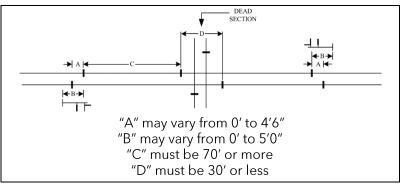
Figure 001-14: Railway Grade Crossing – Double Rail Track Circuit
