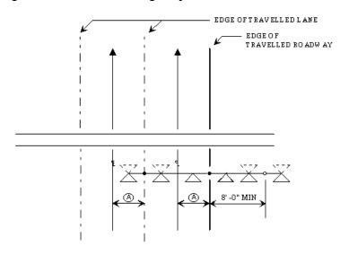
Figure 703-5: Multilane Highway With Curb
