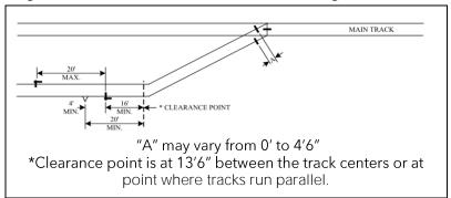
Figure 001-10: Turnout - With Point Derail
