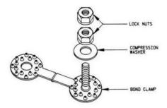
The C-2085 bond stud coin consists of four parts: a 11.2. perforated sandwich-type bond clamp with a threaded stud. One compression washer and two securing locknuts. Specially designed tangs pierce the thin polyolefin film which coats the screen.
