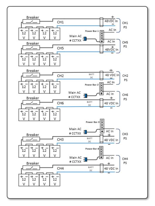
Figure 9: Radio System Battery Diagram
