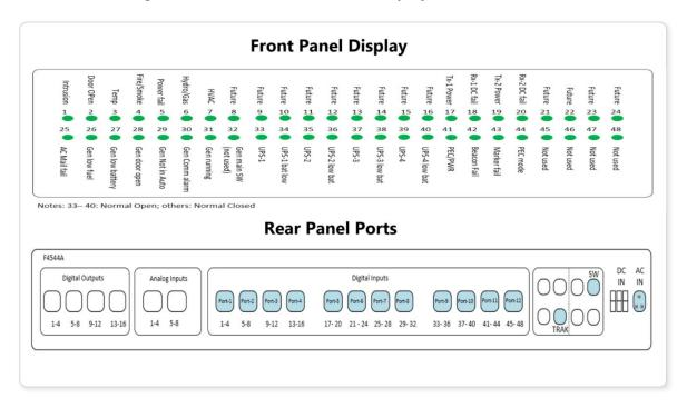
Figure 14: SDM3000 LED Panel Display, Rear Panel Ports
