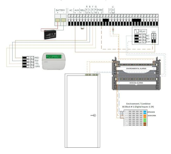
Figure 13: MOSCAD alarm panel
