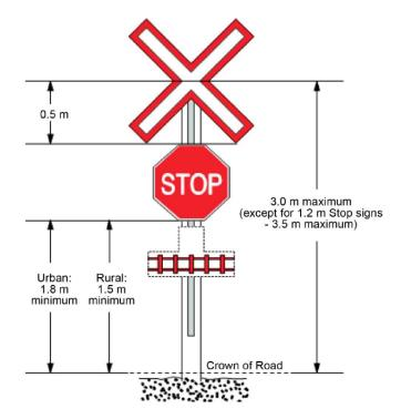
FIGURE 11-6: STOP SIGN PLACEMENT (TRANSPORT CANADA, 2019)
