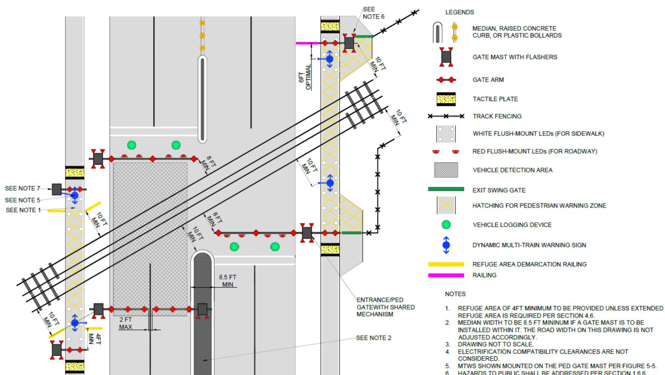
FIGURE B-5: GRADE CROSSING ENHANCEMENTS GENERAL ARRANGEMENT – ACUTE ANGLE
