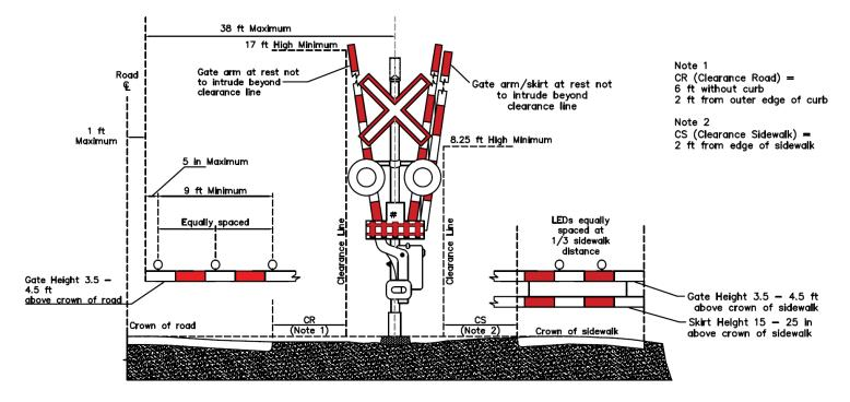
FIGURE 4-3: PEDESTRIAN & ENTRANCE GATE WITH SHARED MECHANISM
