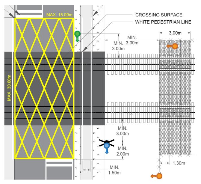
FIGURE 11-2: CROSSHATCHING AND PEDESTRIAN GUIDELINES
