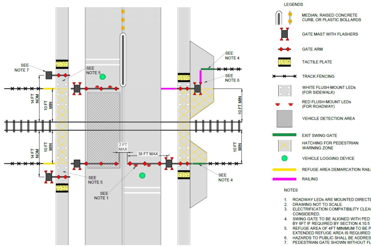
FIGURE B-4: GRADE CROSSING ENHANCEMENTS GENERAL ARRANGEMENT – PERPENDICULAR
