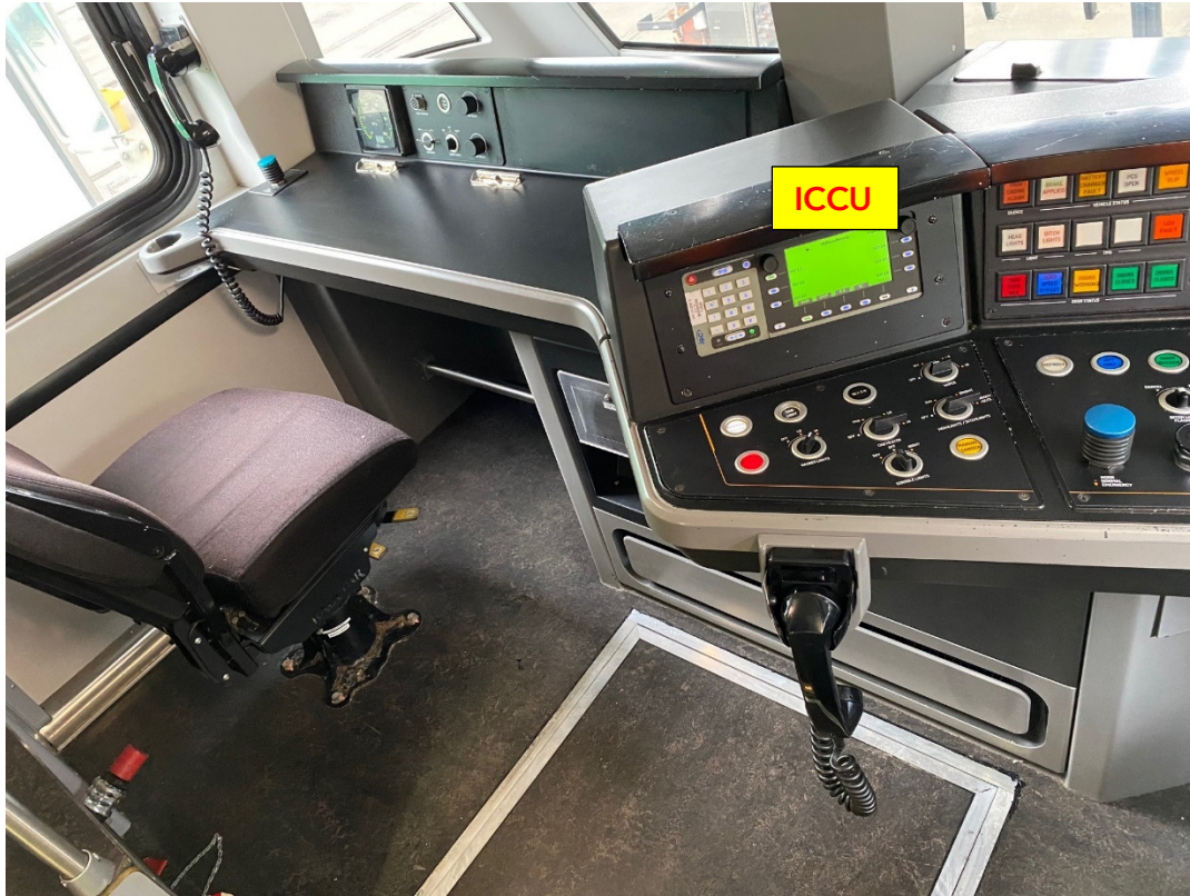
Figure 2: Locomotive ICCU layout
