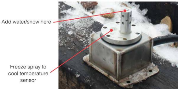
Figure 611(b)-01 Ground Sensor
