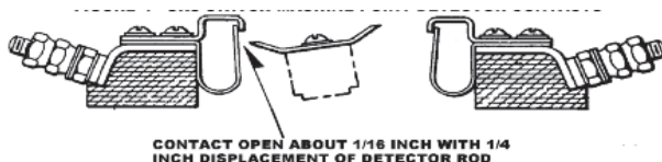
Figure 329(b)(2)-06: GRS Switch Machine Point Detector Contacts.
