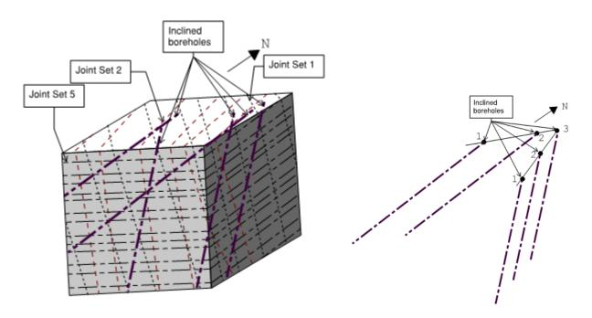
Figure 27 Sample Bedrock Block Diagram - A Cluster of Testing Boreholes
