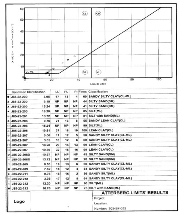
Figure 12 Example Atterberg Limits Test Results
