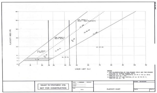
Figure 11 Bank Atterberg Limits Test Results
