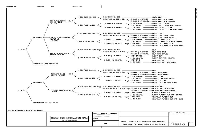
Figure 13 (C1) Flow Chart for Classifying Fine Grained Soil (50% or More Passes No. 200 Sieve)
