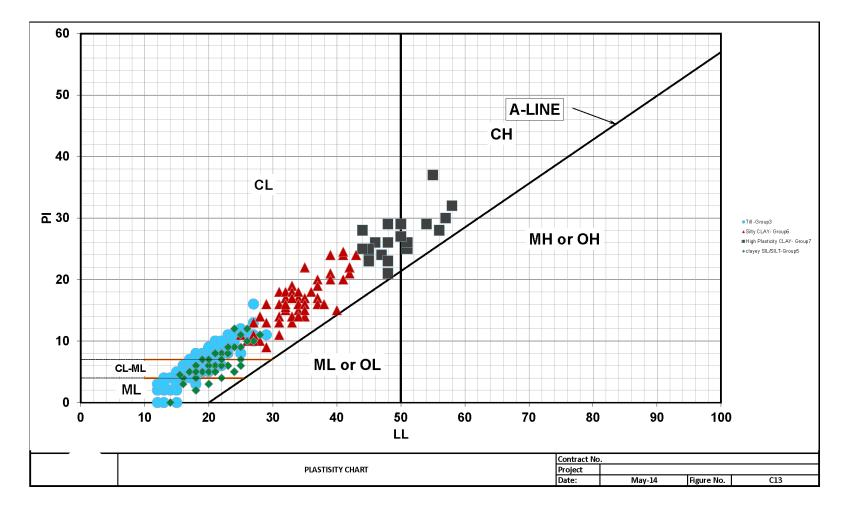
Figure 25 (C13) Atterberg Limit Envelopes for Plastic Soils
