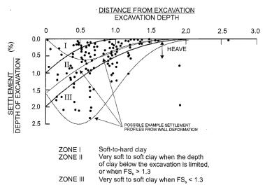
Figure 4 Settlements Adjacent to Excavations in Soft to Medium Stiff Clay (from CFEM)
