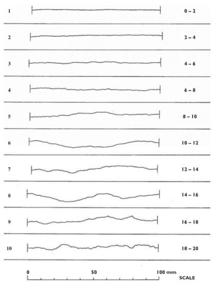
Figure 29 Typical Roughness Profiles for JRC (Bandis et al, 1983)
